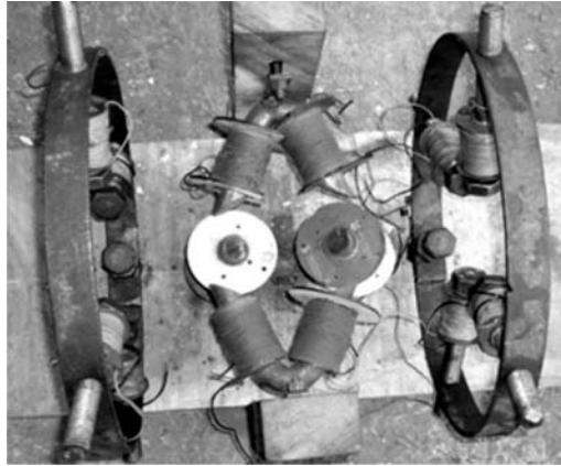
Fig. 6(a). The complete assembled stator part.
