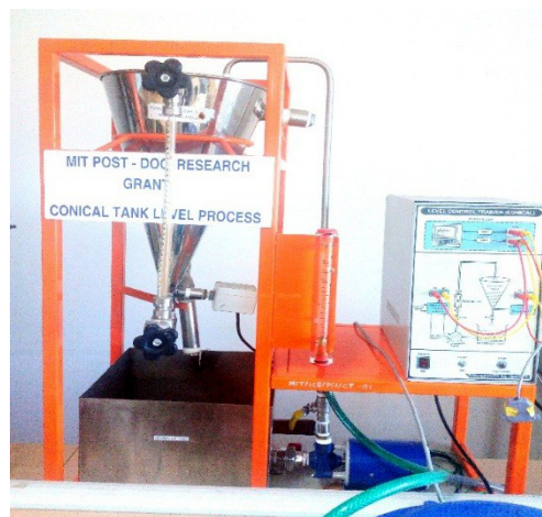
Figure 1: Experimental setup of conical tank
