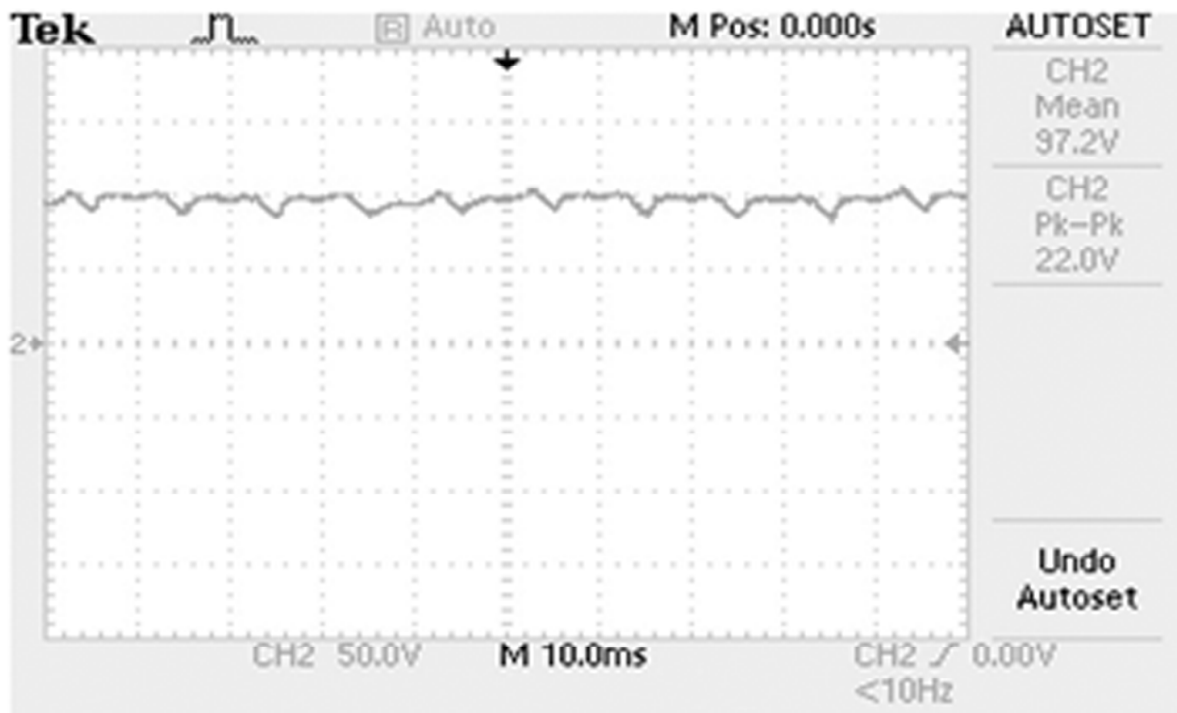
Figure 9: Output of the single stage boost rectifier
