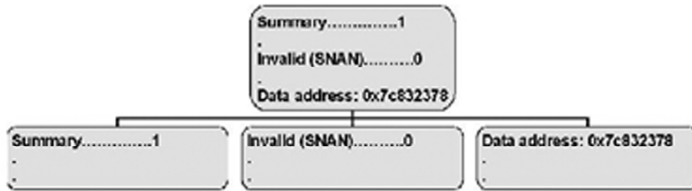
Figure 4: IPLoM Step 1: partition by event size. Separates the messages into partitions based on their event size.
