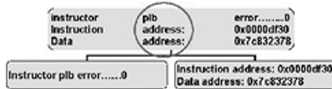
Figure 5: IPLoM Step 2: partition by token position. Selects the token position with the least number of unique values, token position 2 in this example. Then, it separates the messages into partitions-based unique token values, i.e., “plb” and “address:”, in the token position.
