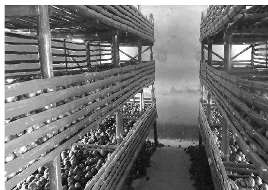
Picture 1: Bamboo racking system
