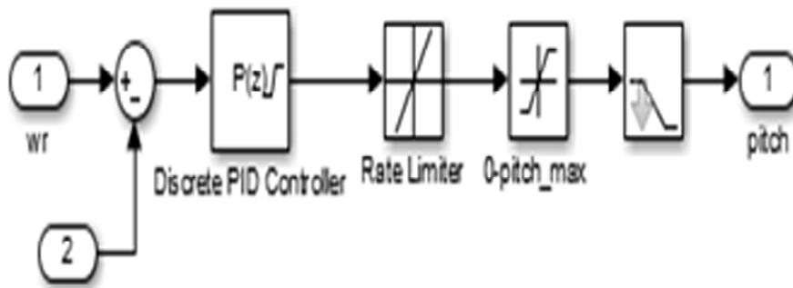
Figure 3: Pitch angle controller
