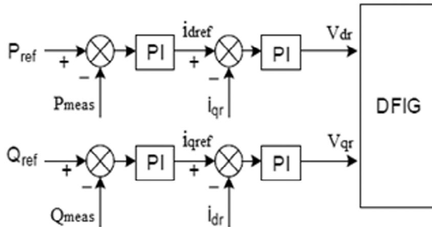
Figure 5: Rotor side converter control
