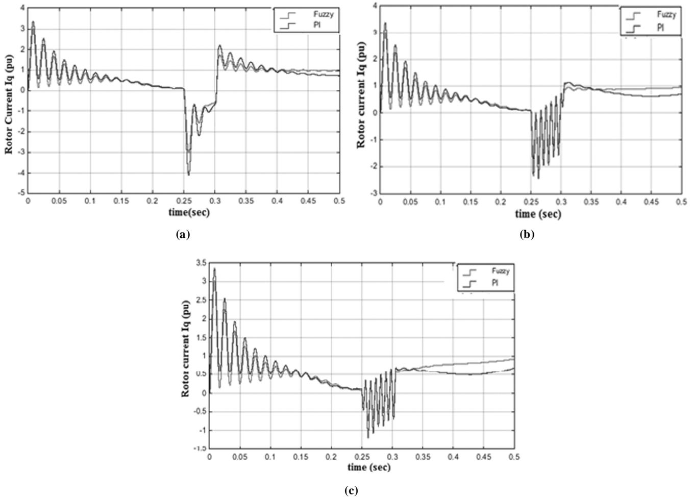
Figure 18: Rotor Current  $I_q$  with PI & Fuzzy Controllers along with crowbar for a (a) three-phase fault, (b) double-line to ground fault & (c) single-line to ground fault
