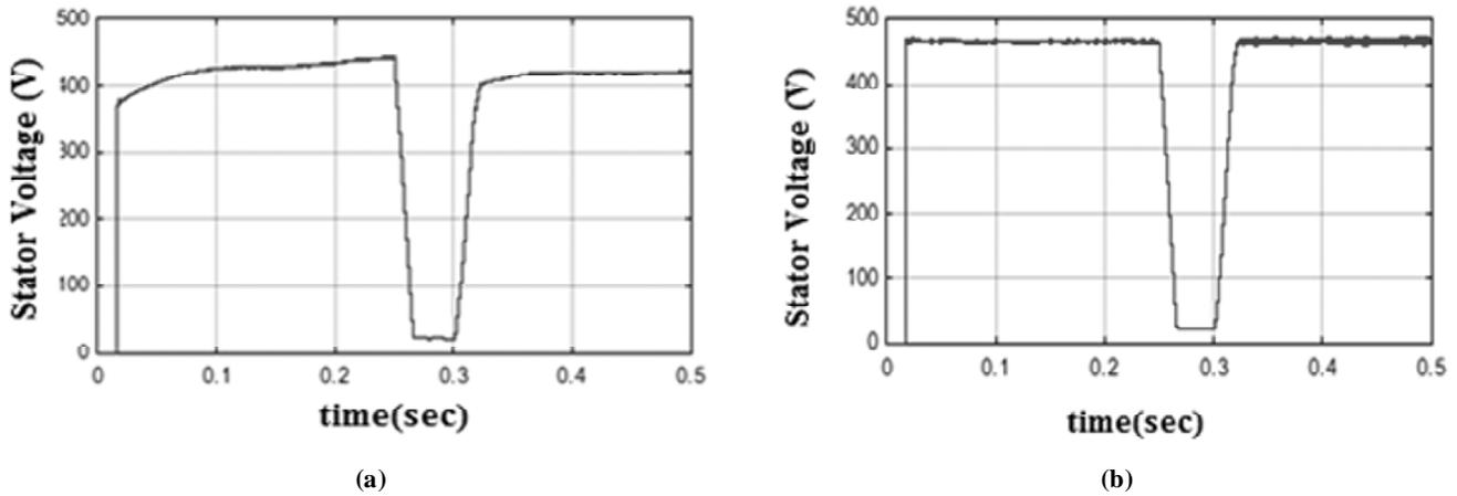
Figure 11: Stator Voltage dip (a) without crowbar (b) with crowbar
