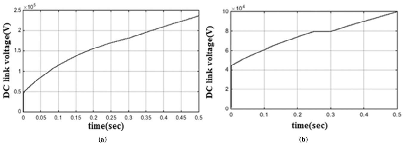
Figure 15: DC link voltage (a) without crowbar (b) with crowbar protection
