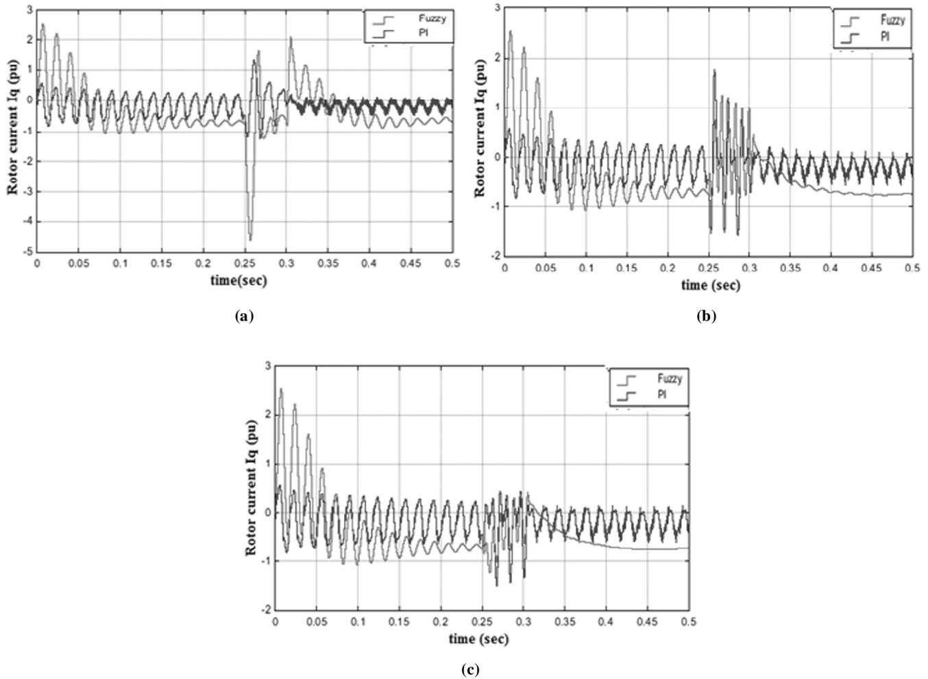
**Figure 21: Rotor Current  $I_q$  with PI & Fuzzy Controllers along with crowbar for a (a) three-phase fault, (b) double-line to ground fault & (c) single-line to ground fault**
