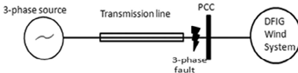
Figure 9: Single line diagram of the test system
