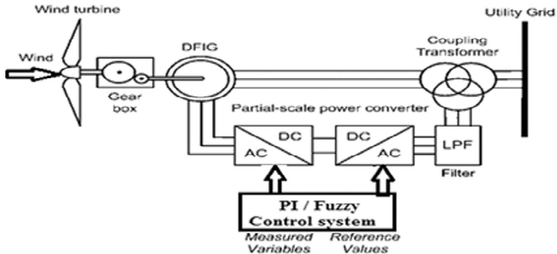
Figure 1: Basic line diagram of a DFIG wind turbine connected to grid
