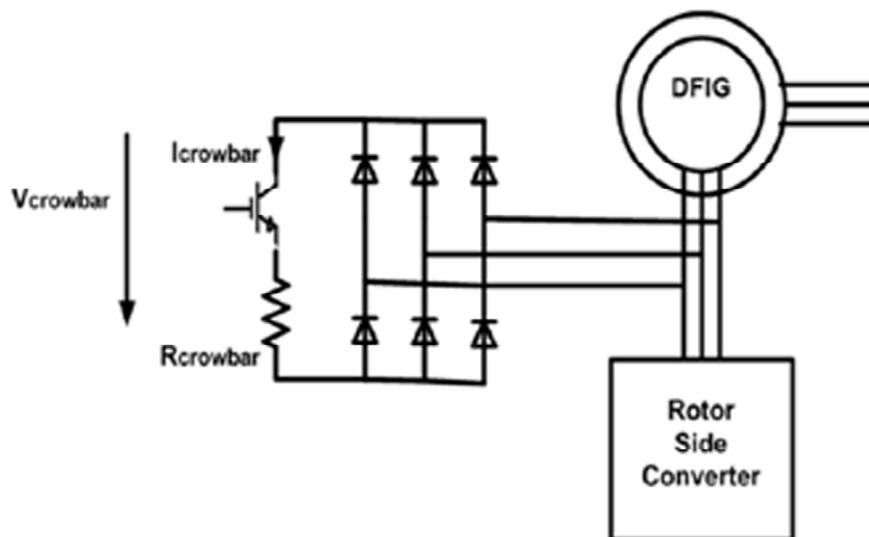
**Figure 7: Connection of crowbar in the rotor circuit**
