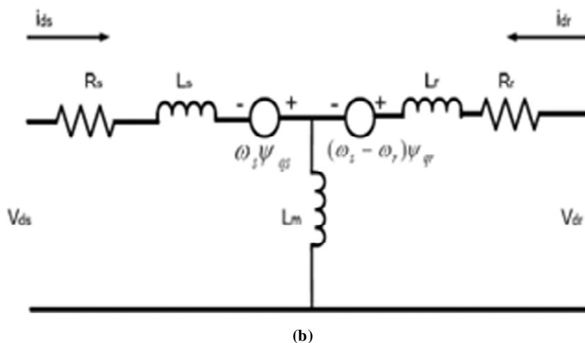
Figure 2: (a), (b). Equivalent circuit of DFIG in dq-reference frame
