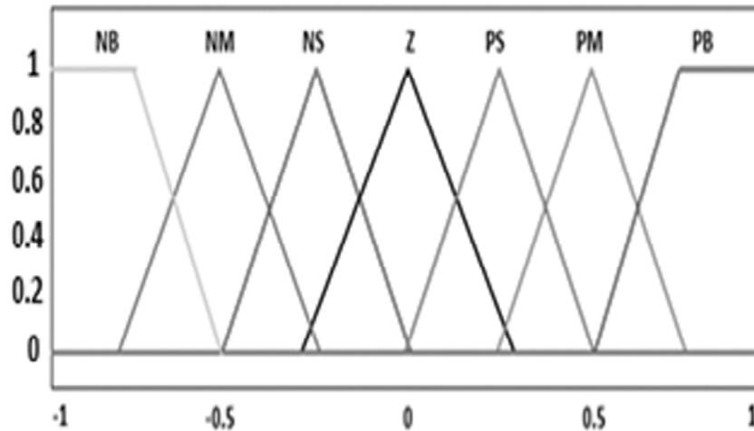
Figure 8: Membership functions for input & output signals
