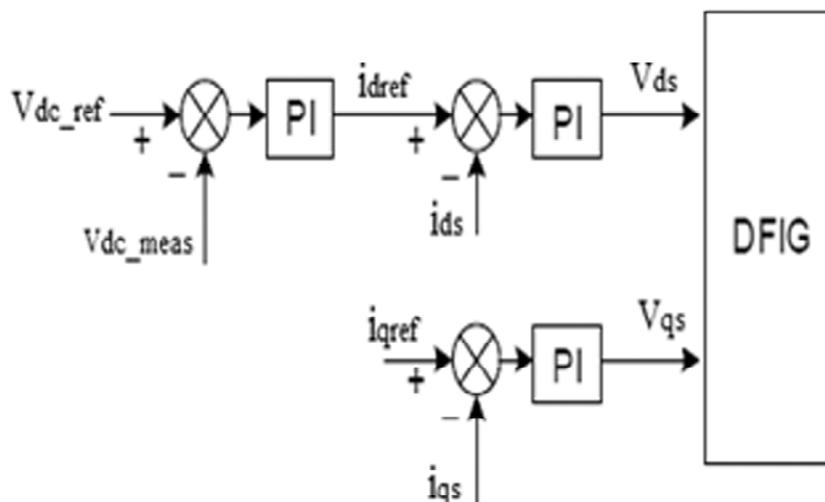
Figure 4: Stator side converter control
