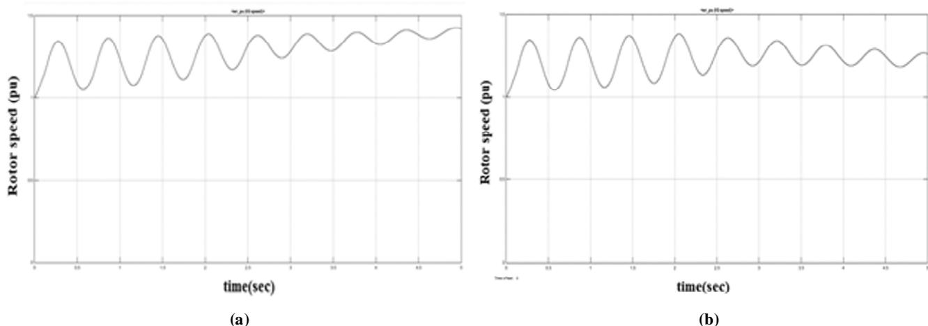
Figure 10: Rotor speed during grid fault (a) without pitch angle controller, (b) with pitch angle controller
