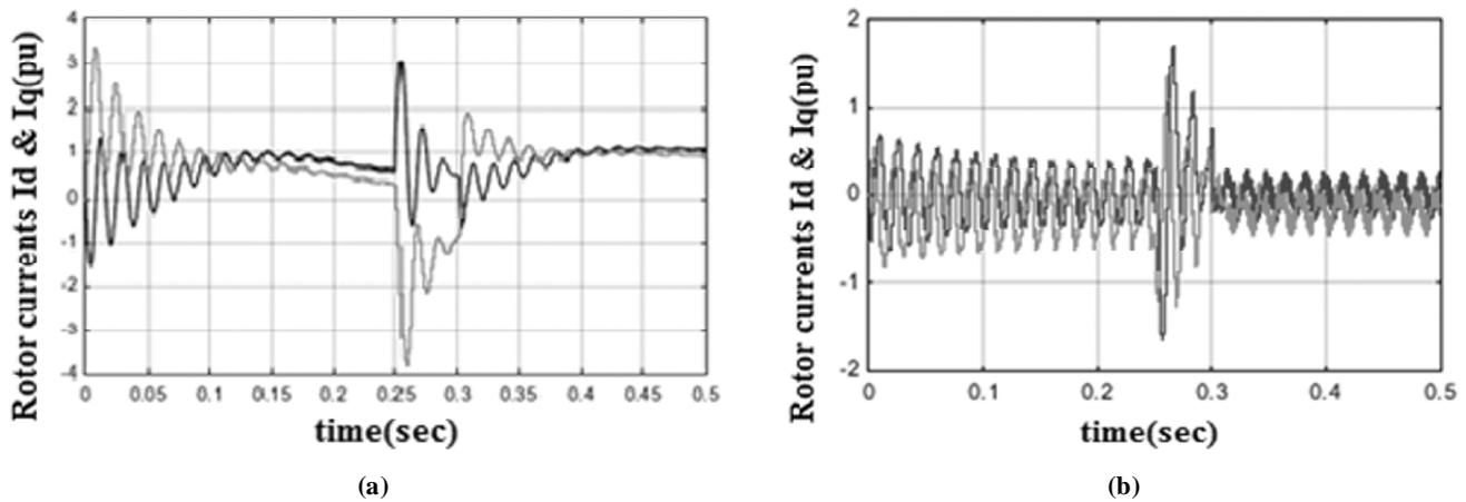
Figure 12: Rotor Currents Id & Iq (a) without crowbar (b) with crowbar
