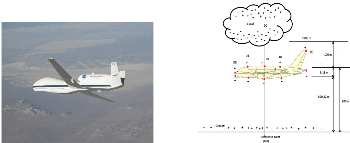
Figure 1: (a) NASA Global Hawk (Aviation Instrument Technologies Inc) Devoted to Lightning Research. (b) Dipole placements along the aircraft surface [6]
