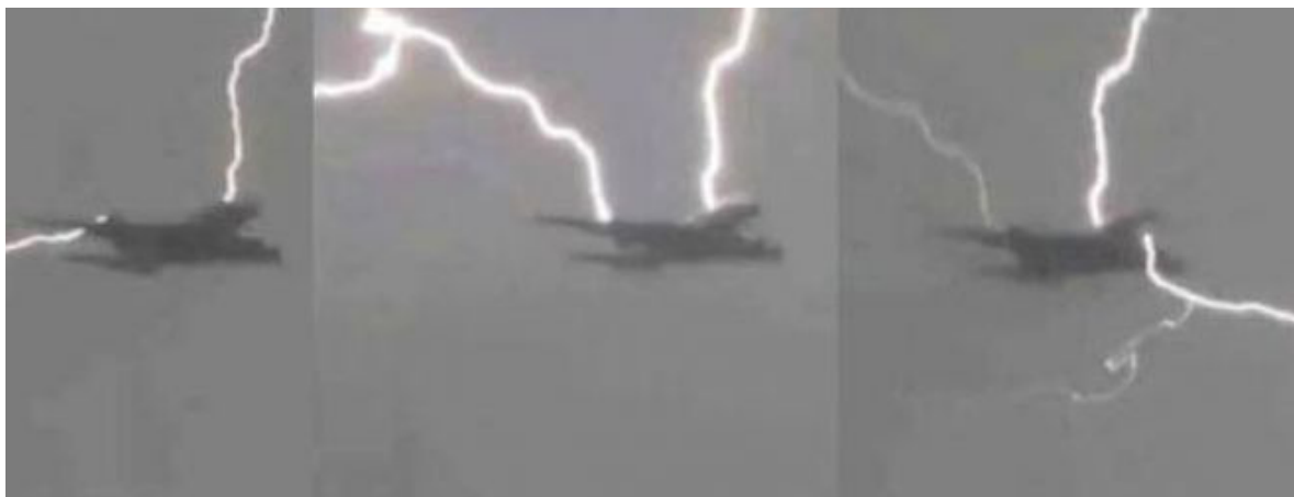
Figure 3: An A380 aircraft stuck at Heathrow airport: showing swept stroke as the aircraft moves with respect to the thundercloud (dailytelegraph.co.uk)
