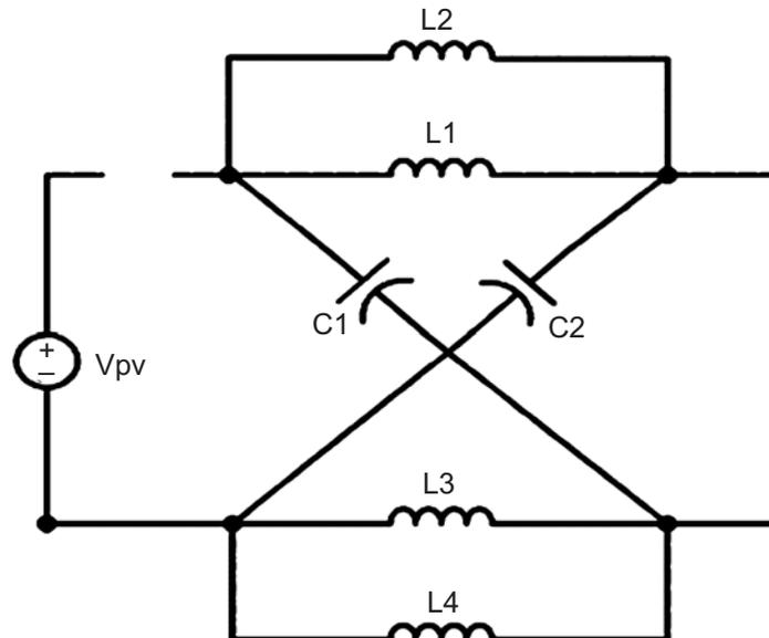
Figure 7: Equivalent circuit for shoot through state
