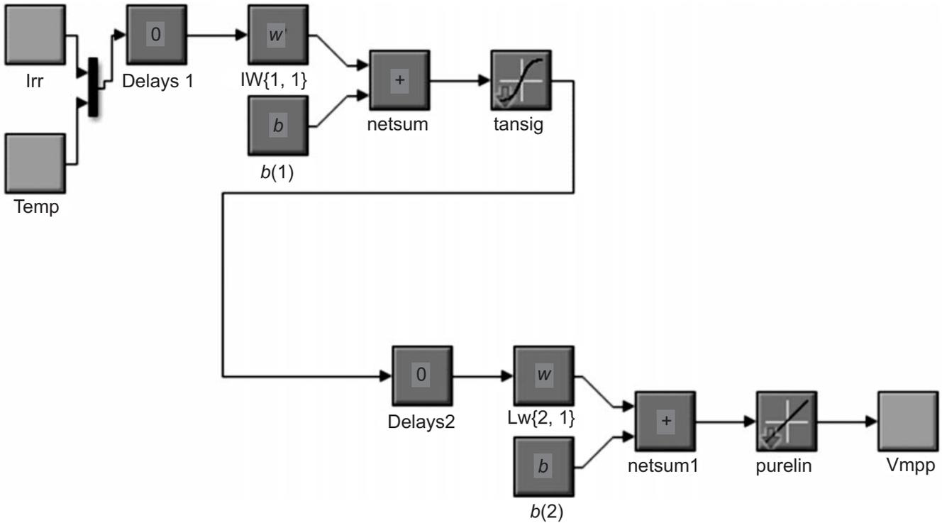
Figure 5: Matlab/Simulink model of ANN
