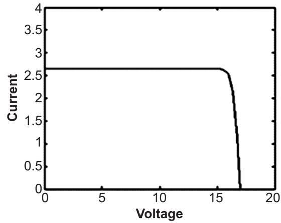
Figure 10: I-V curve for a PV cell
