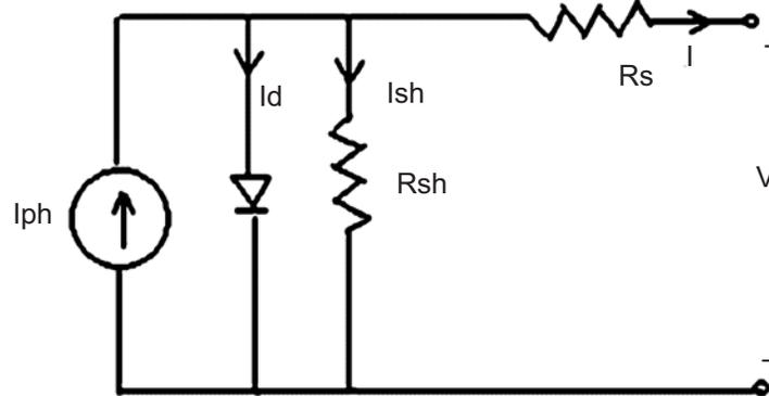
Figure 2: Equivalent circuit of Photovoltaic cell
