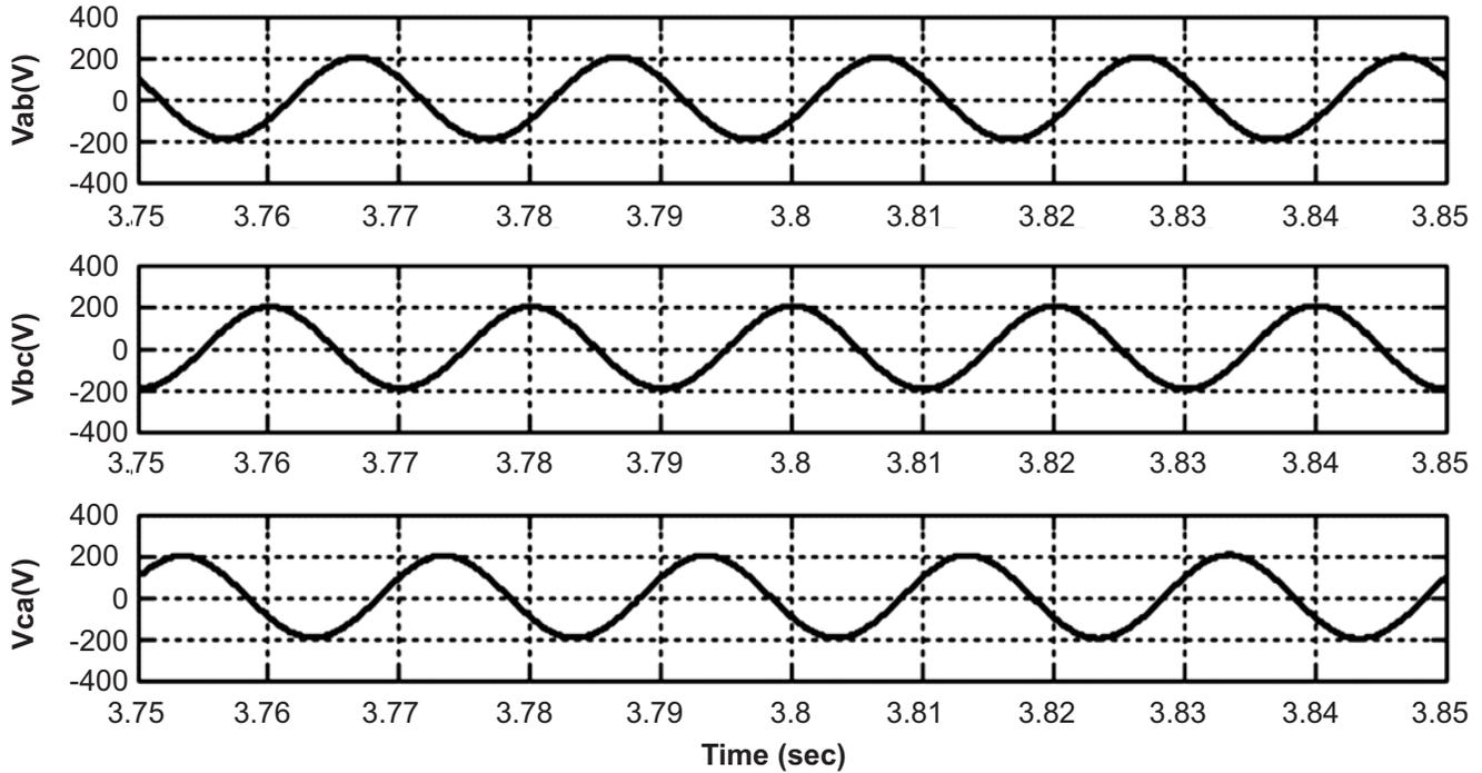
Figure 17: SL-ZSI output voltage with resistive load
