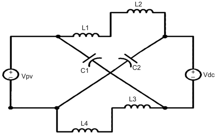
Figure 8: Equivalent circuit for Non shoot through state of SL-ZSI
