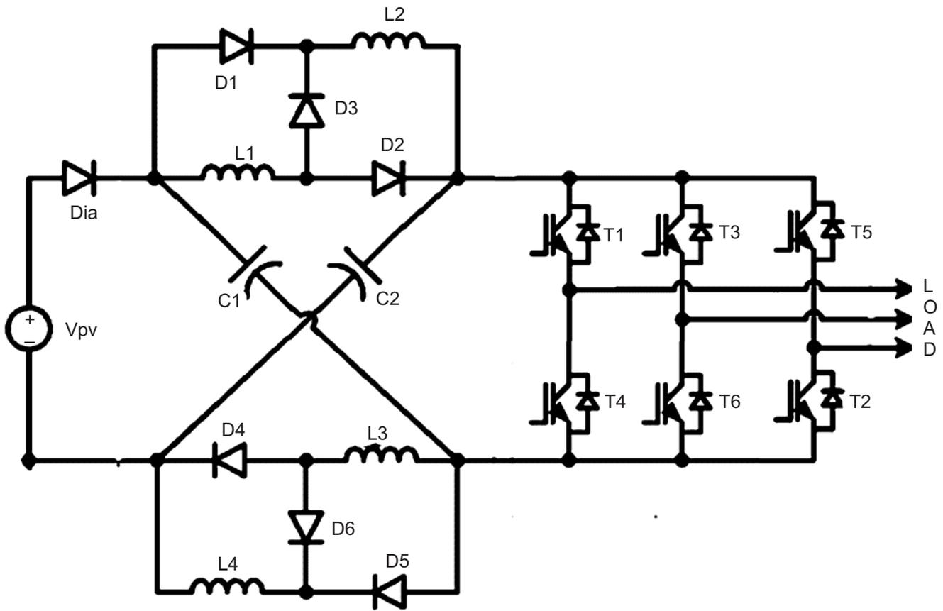
Figure 6: Equivalent circuit of [SL] ZSI
