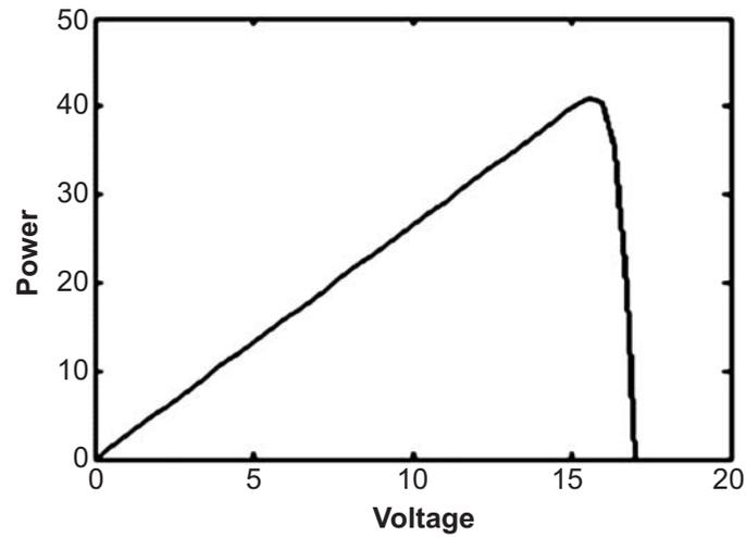
Figure 11: P-V curve for a PV cell
