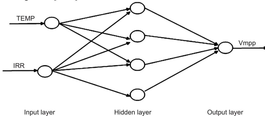
Figure 3: Neural network for Back propagation algorithm
