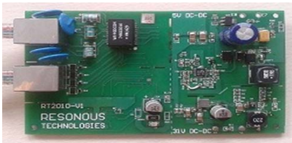
Figure 8. PCB OF POE PD DEVICE.
