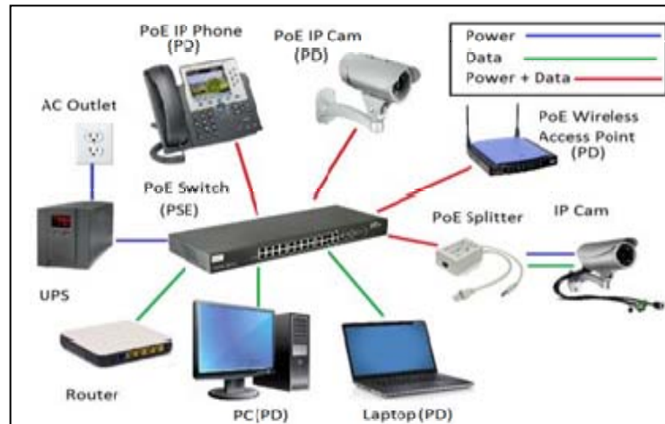
Figure 1. Typical PoE System
