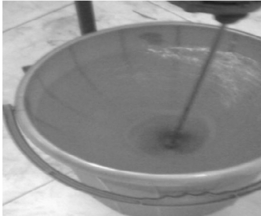
Figure 1: Mixing of Al_2O_3 nanoparticles to water
