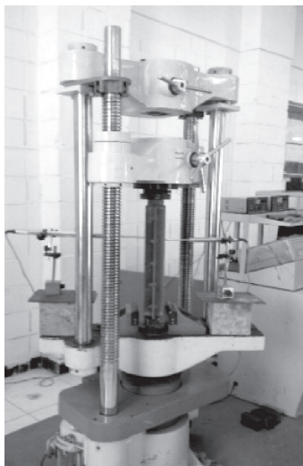
Figure 1: Concrete in-filled light steel gauge column
