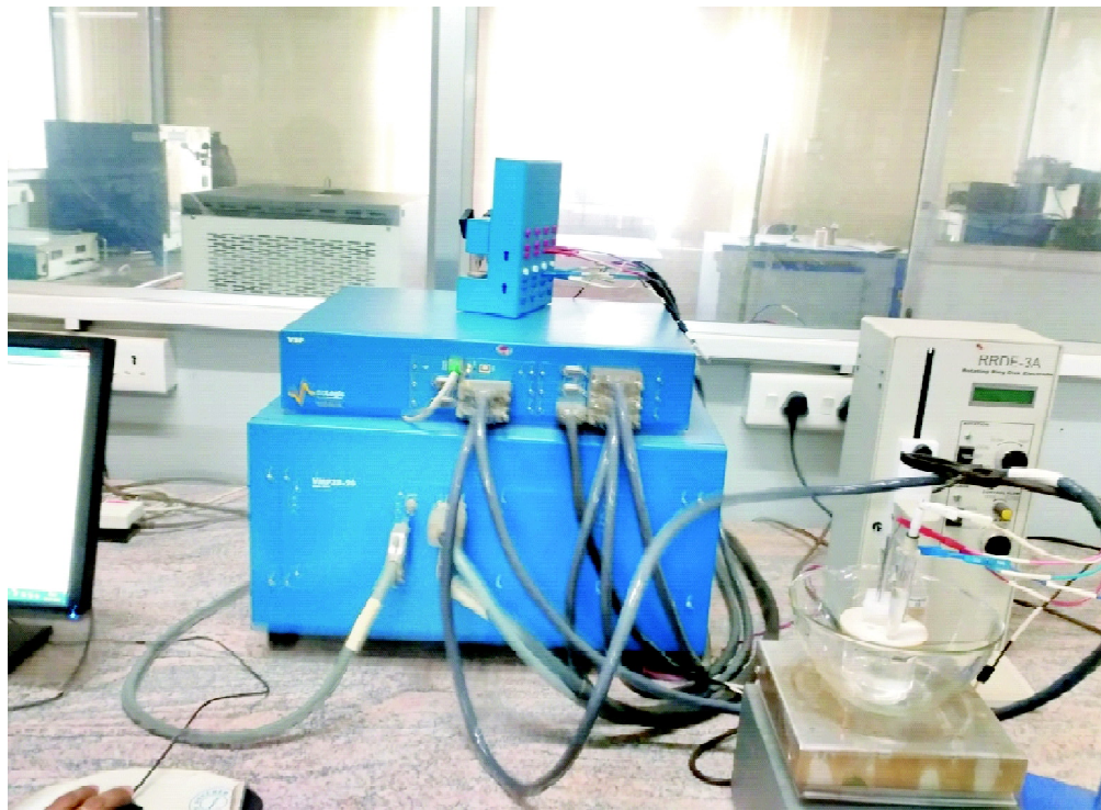
Figure 4: Electrochemical workstation connected to cell
