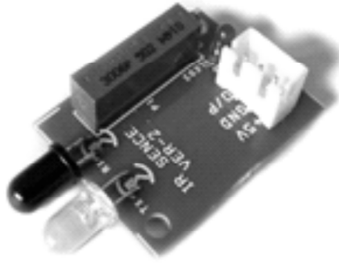
Figure 2: Infrared Sensor -B PID Control System
