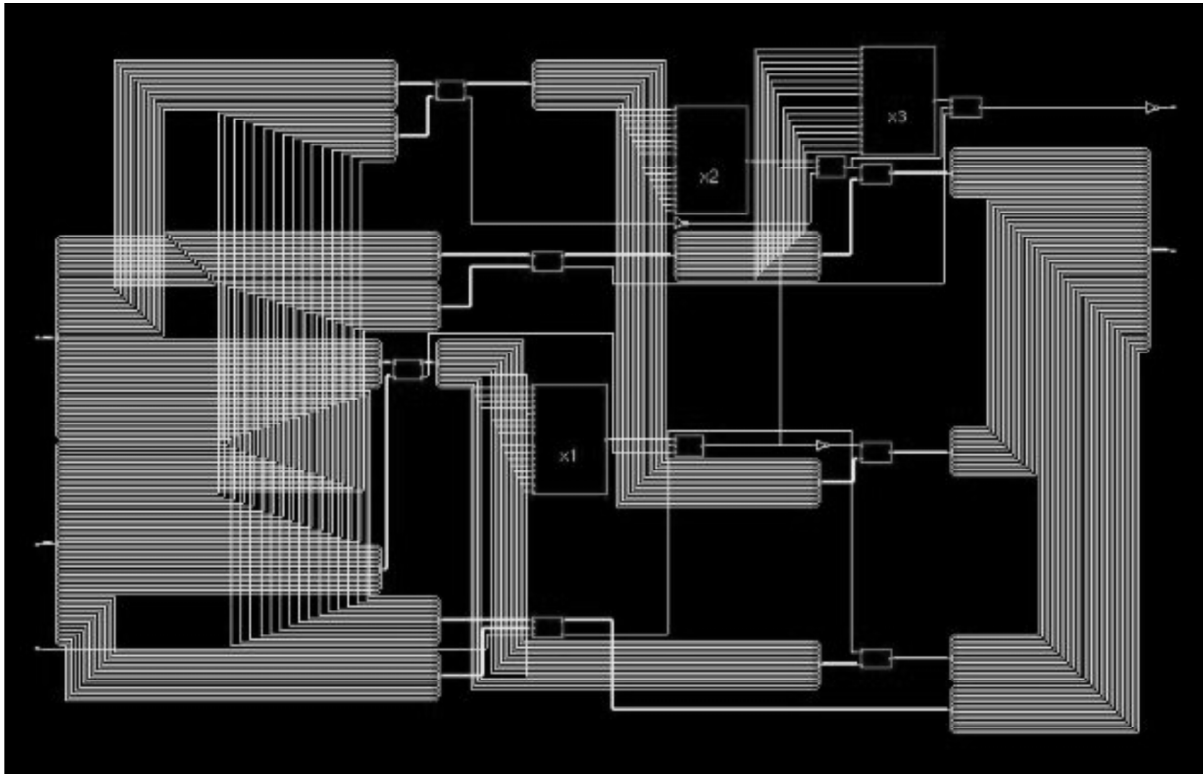
Figure 6: Gate level net-list of concatenation and incrementation carry skip adder
