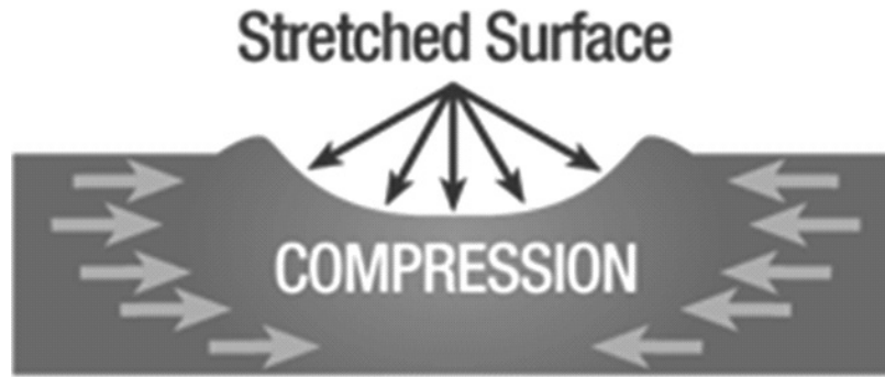
Figure 6: Tensile Stress Corrosion
