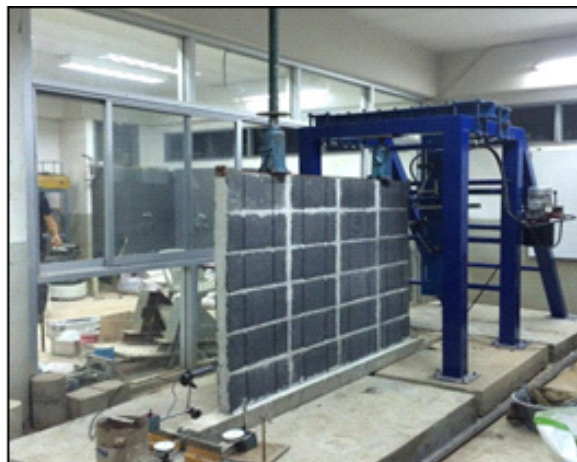
Figure 3: Test set-up for concrete block walls
