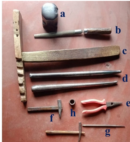
Figure 2- Instruments used for manufacturing of Brass Craft: (a) Hatudi Munda (Hammer Head); (b) Doria Pagara (U- Shaped File); (c) Bikhyani Katha (Wooden T); (d) Matha Sabala (Chisel); (e) Pakada (Forceps); (f) Choto Hatudi (Small Hammer ); (g) Ugha (File); (h) Bolta (Bolt).
