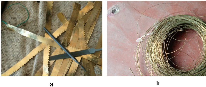
Figure 4- Raw materials for brass craft making (a. Copper sheet and b. Copper wire).
