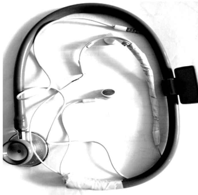
Figure 2: Smart stethoscope designed from conventional stethoscope
