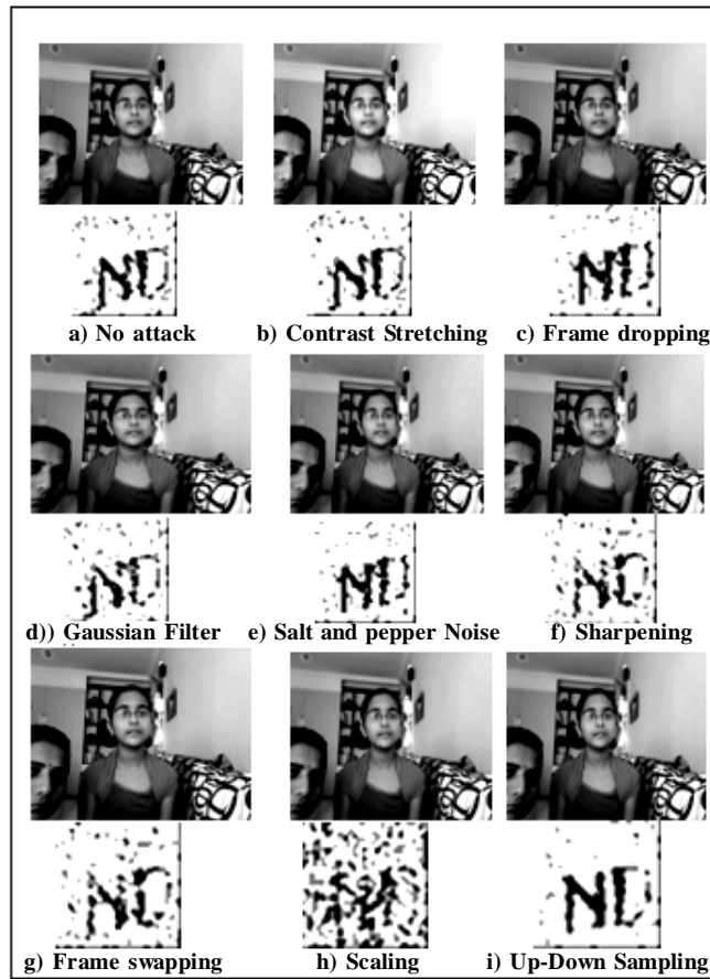
Figure 12: Attacked Frames and Extracted Watermarks of Log Gabor Based FFT Watermarking
