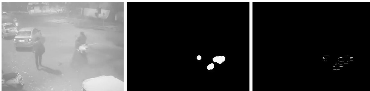
Figure 3: Normal activity frame, corresponding foreground motion disks and optical flow vectors
