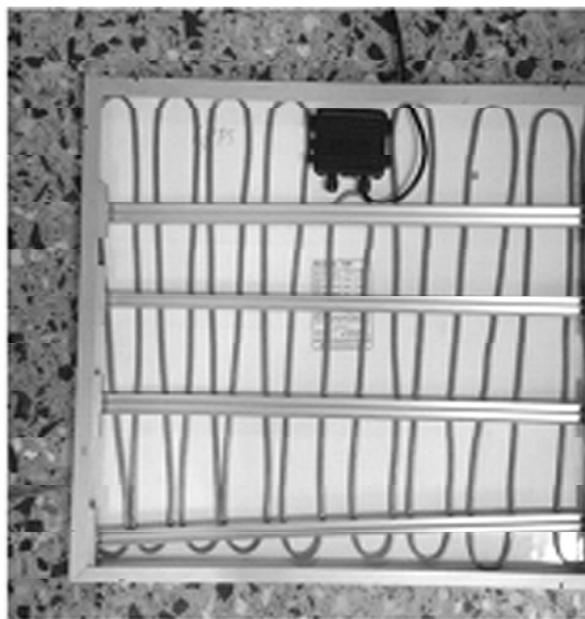
Figure 4.2 completed test model of PV system with cooling tubes
