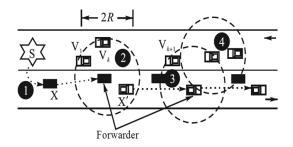
The above two mechanisms cannot guarantee the waiting time the tail vehicles in a cluster encountering the reverse forwarders. In particular, there is a longer delay when the DSRC devices have a lower popularity rate.
