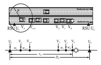
According to the experimental data in the reference [11], the vehicle density obeys the exponential distribution. The distance between two driving vehicles along the eastbound road can be represented by the vehicle density  $\lambda e$ . The number  $N_e(r_U)$  of vehicles in the interval  $r_U$  (the distance between the source vehicle and the rear first RSU) obeys a Poisson distribution.
