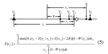
Here the  $x_w$  is the distance from the covering range of the last vehicle in the source vehicle cluster to the X. The distance between the vehicles in the westbound road
