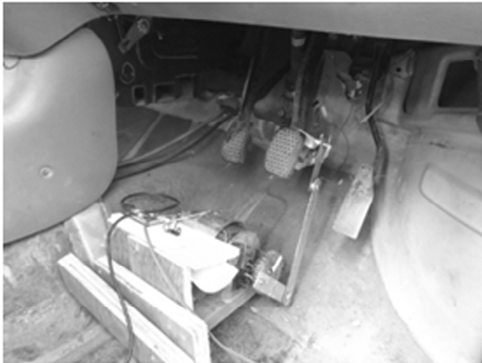
Figure 6: Hardware of the braking unit
