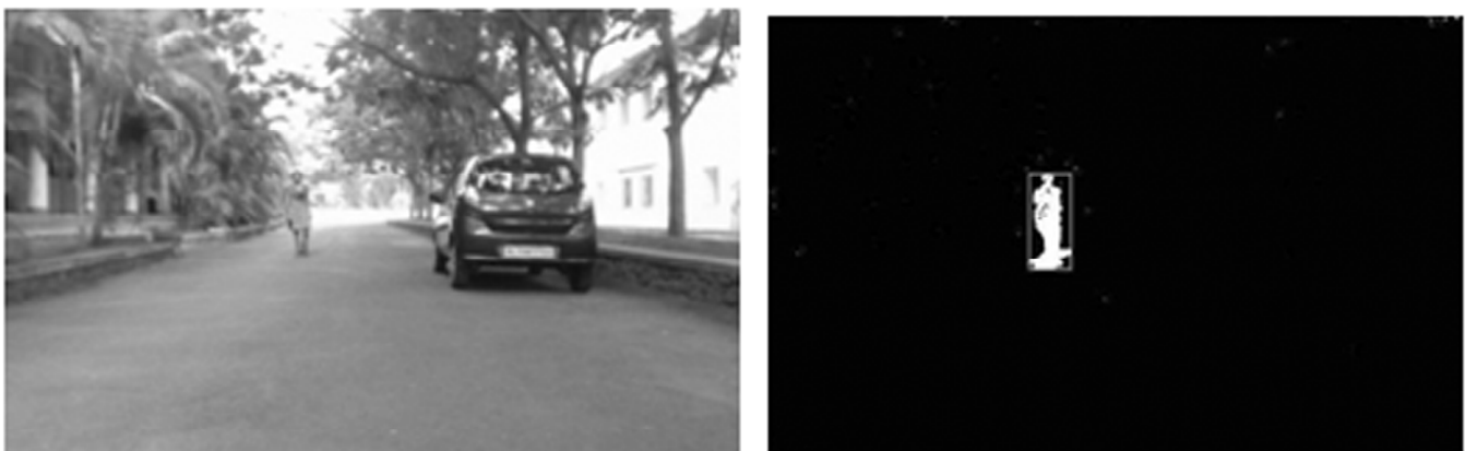
Figure 4: Blob analysis performed over the foreground pixels. The rectangle represents detected pedestrians.
