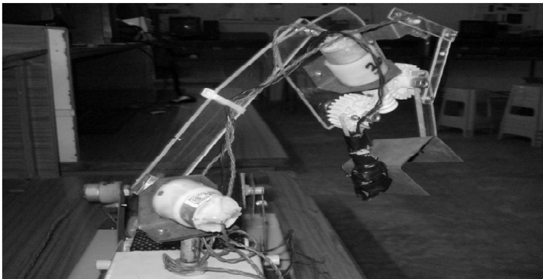
Figure 7: Robotic arm picking an object and moving away from the conveyor
