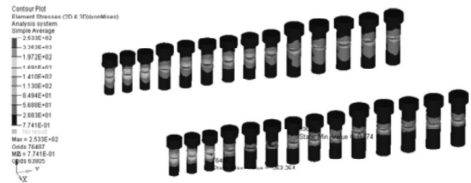
Figure 9: Von-mises Stress Contour on Bolts
