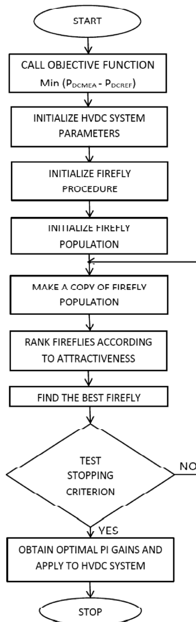
Figure 6: Flowchart for Minimization of the Rectifier/the Inverter DC Power Error Function using Firefly Algorithm
