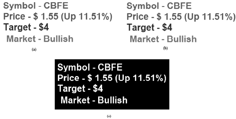
Figure 6: (a) Original Image, (b) Gray Scale Image, (c) Binary Image
