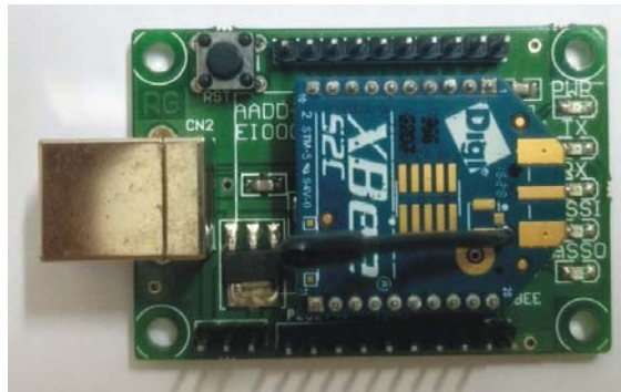
Figure 13: The receiver module (base station) with XBee shield which can be easily interfaced with a data logging and computing device with an USB cable.
