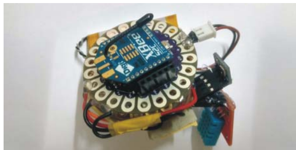
Figure 12: Arduino Lilypad XBee Module (for transmission) coupled with the microcontroller and attached to BMP180 and DHT11 sensors
