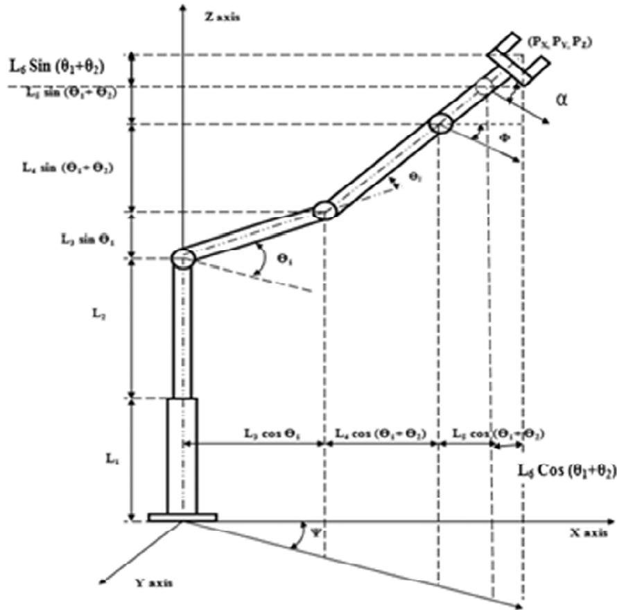
Figure 3: Geometric structure of the robot
