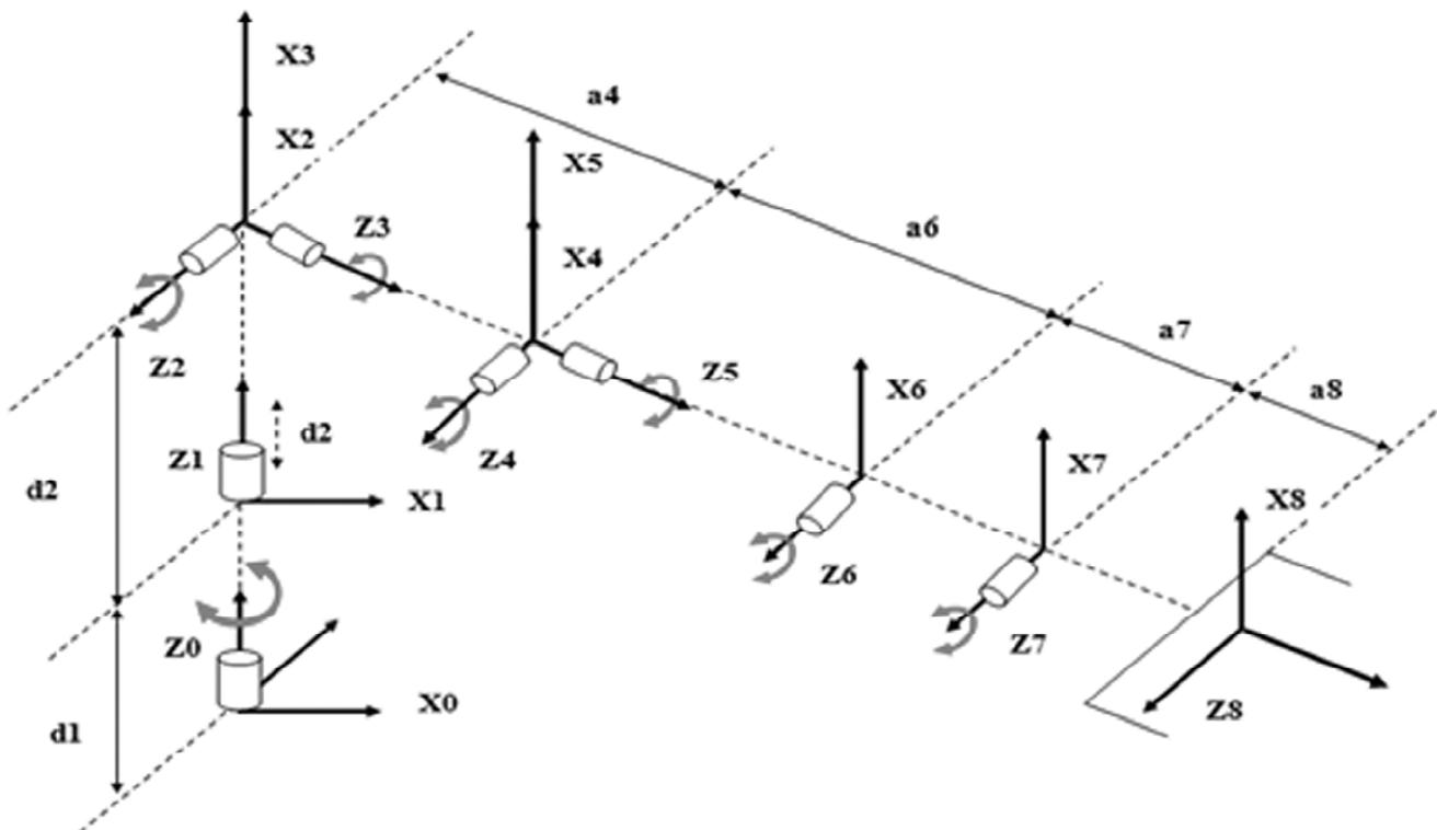
Figure 2: Part co-ordinate system of the robot
