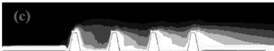
(b) (a) Variation of Nusselt number with duct Reynolds number as function of Prandtl number of the fluid; expanded and cutaway view of (b) temperature contour for Pr = 15 (c) temperature contour for Pr = 0.7.
