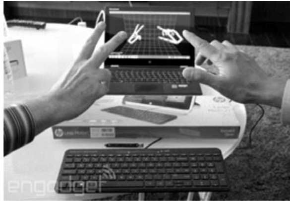
Figure 1: Interfacing of leap motion sensor with PC
