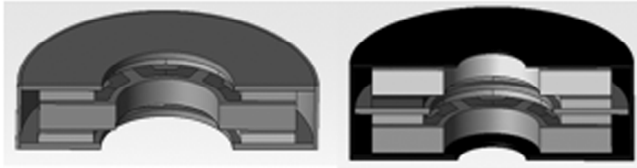
Figure 6: Design Concept on Double Rotor Single Stator & Double Stator Single Rotor
