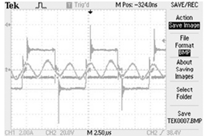
Figure 10: Bridge voltage and inverter current under No- load line regulation at 25VDC input
