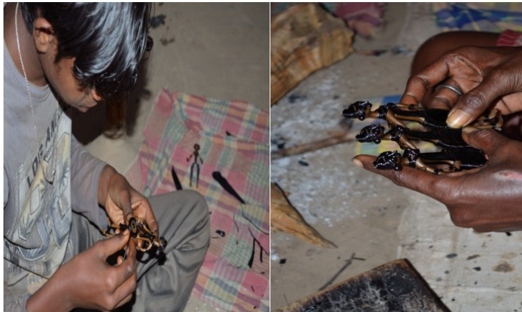
Figure 10 and 11—Formation of the figure with wax, resin and mustard oil preparation
