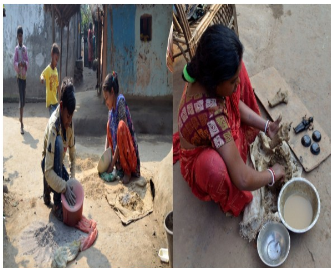
Figure 14 (on the left)—Preparation of soil, ash, sand and clay and Figure 15 (on the right)—First stage of layering
