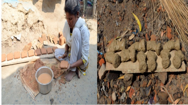
Figure 16 (on the left)—Second stage of layering and Figure 17 (on the right)—Moulds drying after third stage of layering
