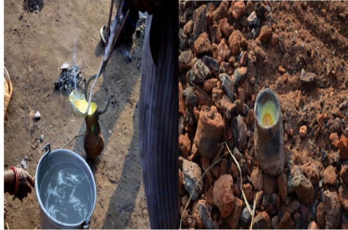
Figure 22 (on the left)—Pouring of melted metal through chong Figure 23 (on the right)—Mould filled with melted metal kept for cooling
