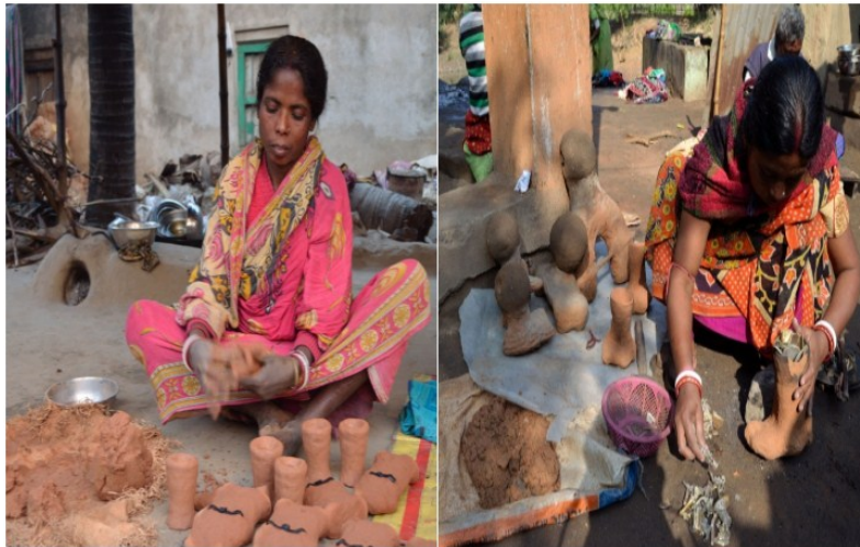
Figure 18 (on the left)—Attachment of funnel-like structure and Figure 19 (on the right)—Covering of funnel-like structure
