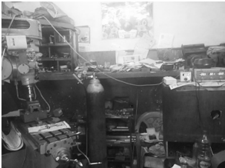
Figure 3: Cryogenic CO 2 Machining Setup
