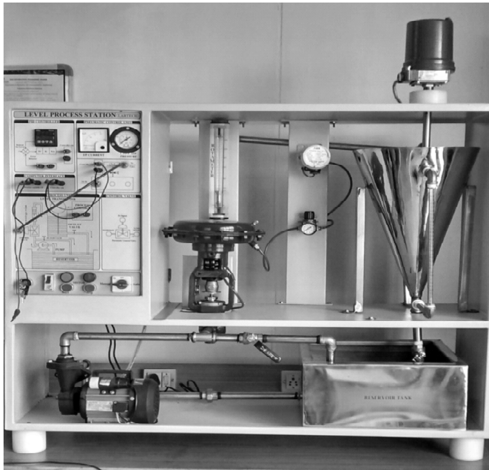
Figure 1: Experimental setup of conical tank system
