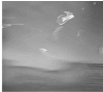
(e) Blur that comes from water splashes is another factor affecting horizon detection.
