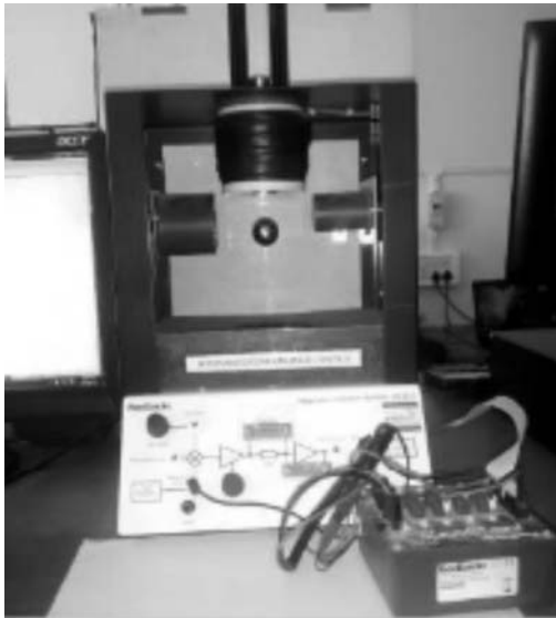
Figure 1: Magnetic levitation system (Feedback 33-210) and its phenomenological model
