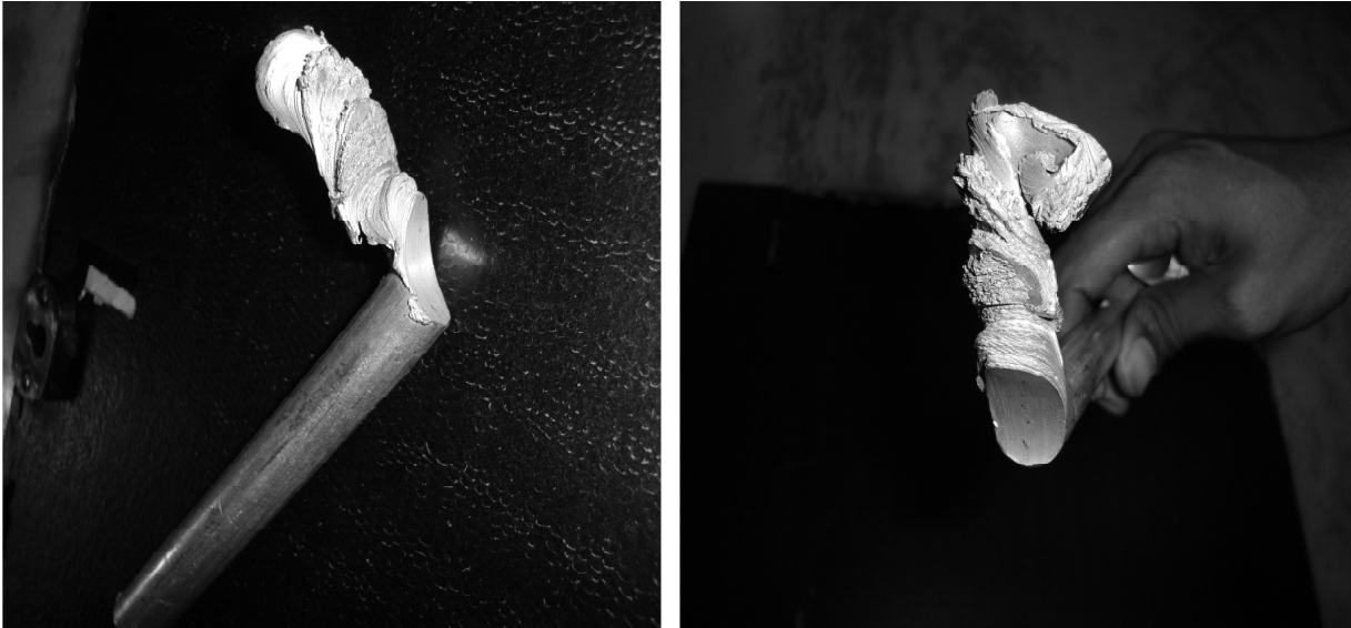
Figure 5: Shows the deformation of the Aluminum mechatrode in friction surfacing process
