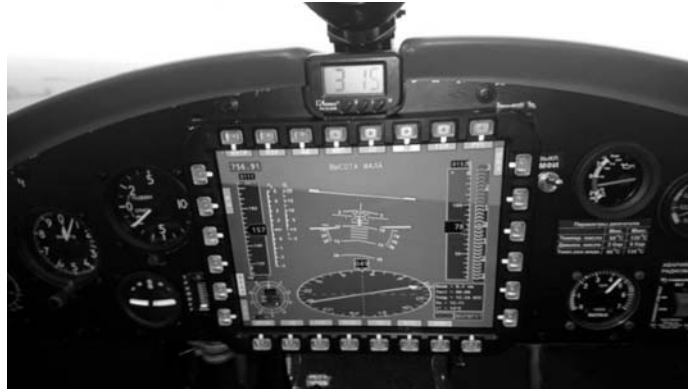
Figure 14: CIISS Display when taking the low altitude
