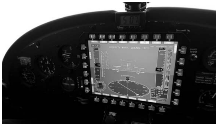
Figure 15: CIISS display when taking the minimum speed
