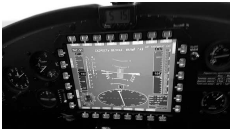
Figure 16: CIISS display when taking the maximum speed
