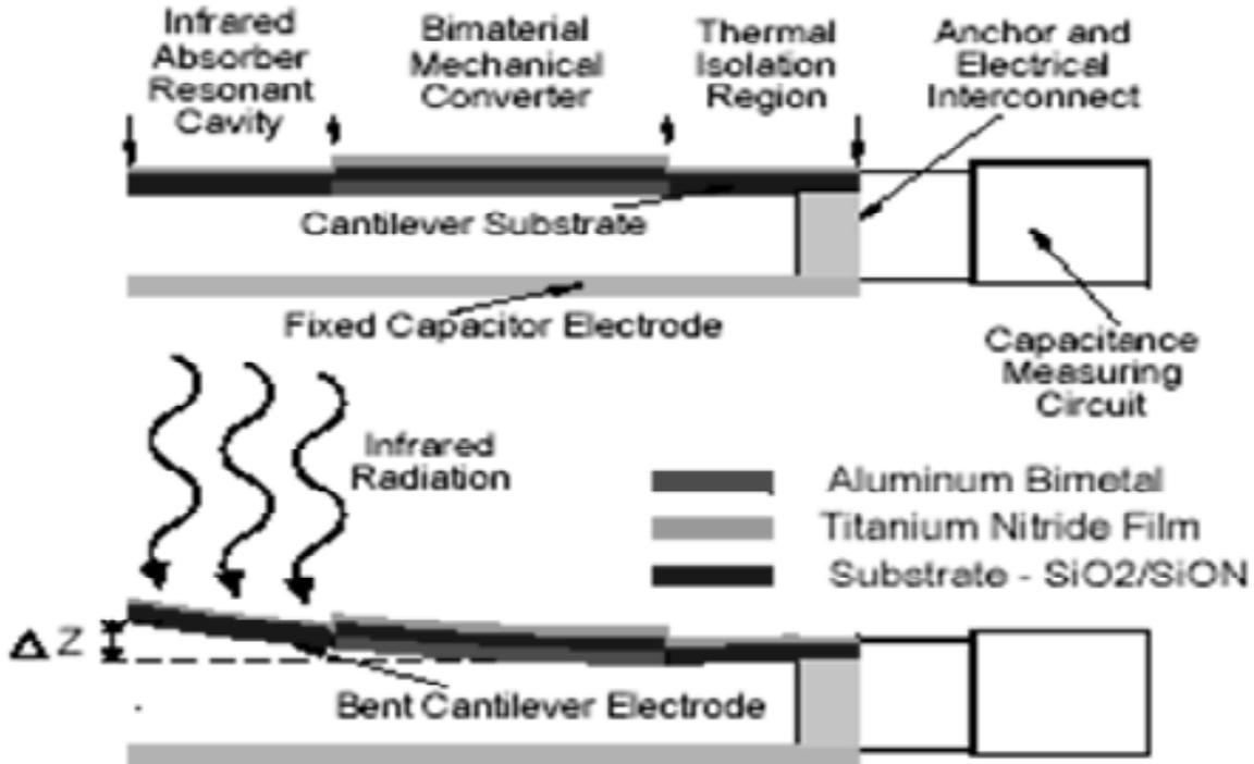
Figure 1: Schematic Diagram Showing the Operating Principle of the Bimorph Microcantilever IR Sensor
