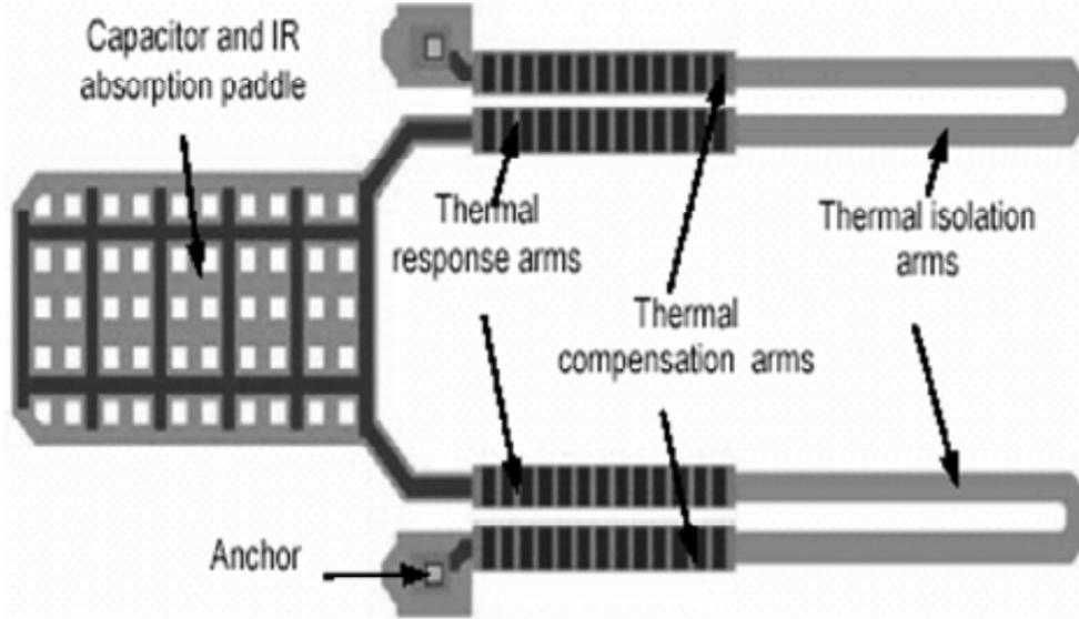
Figure 2: Schematic Diagram of the Thermally Compensated 25  $\mu\text{m}$  Pixel pitch IR Sensor Structure
