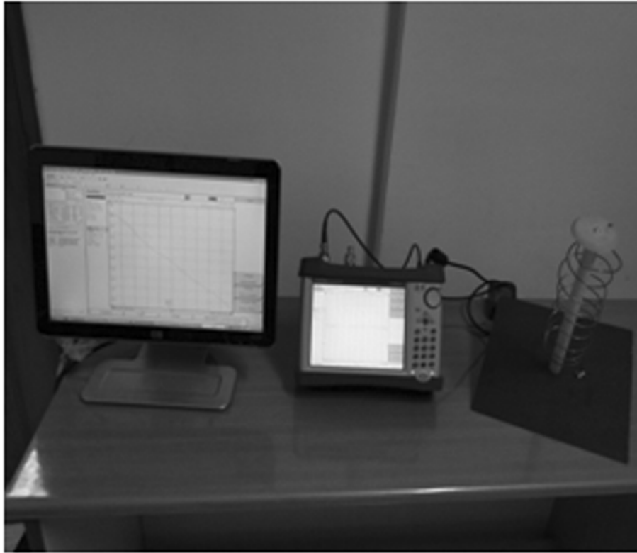
Figure 6: Experimental Setup to measure VSWR
