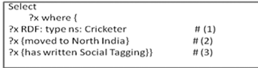
Figure 5: Illustration of the Heterogeneous query model, consists of three patterns, 1) Structure part, 2) Unstructured part, 3) Semi-structured part.
