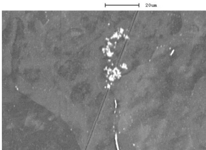
Figure 14: The SEM image of the specimen when applying 160V-magnetic field.
