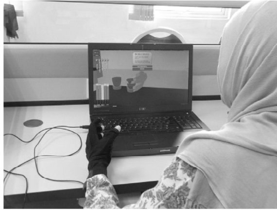
Figure 1 : The 3D Cybertherapy system. The user is wearing a cyberglove connected to the computer
