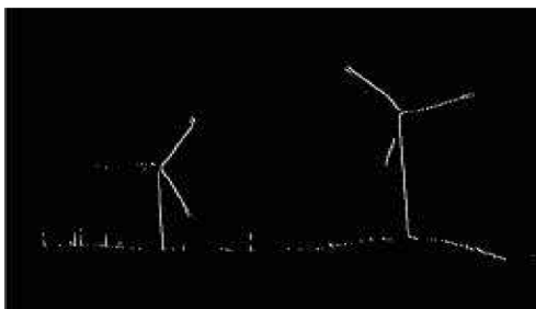
Figure 7: Outputs for edge detection and noise removal
