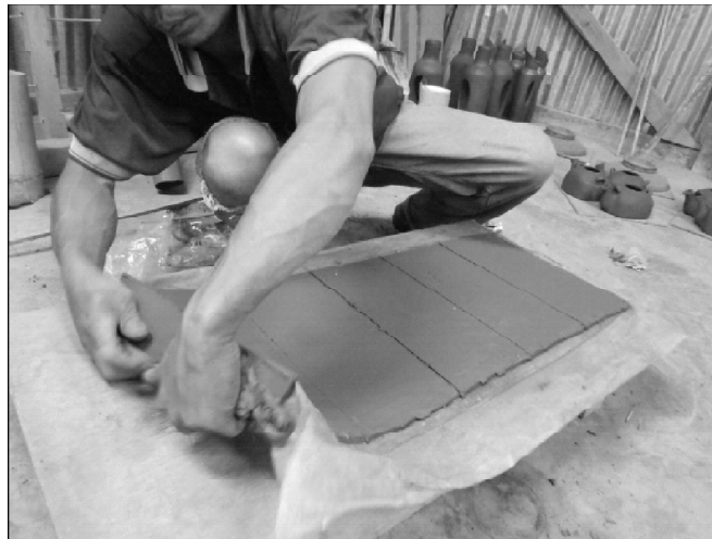
Figure 9: A series of strips are then cut out with the help of a bamboo sliver
