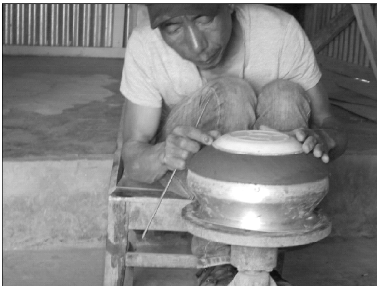
Figure 10: The potter places a strip of clay on an aluminium pot as a base
