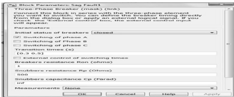
Figure 8: Simulation parameter of single line sag fault
