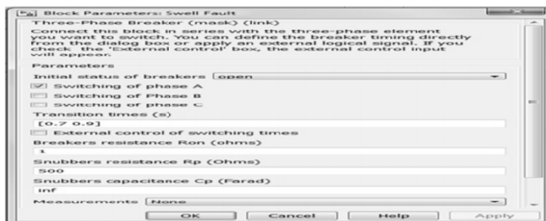
Figure 9: Simulation parameter of single line swell fault
