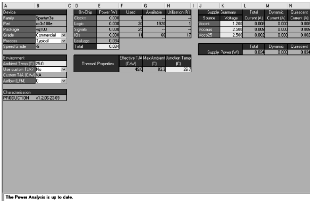
Figure 4: (a) The power calculation of scheme I in [5] (0.034W)
